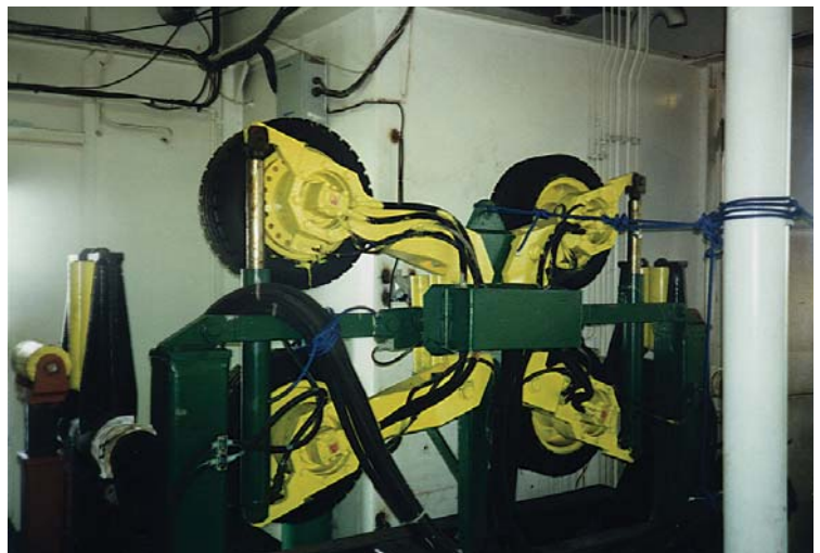
A new type of machine has been developed from Tesmec's existing proprietary technology used for pulling continuous cable.
