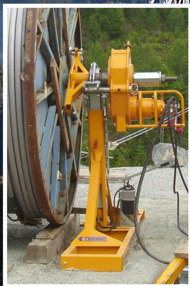
CVI830+TIH013 Hydraulic Drum elevator made of galvanized steel
