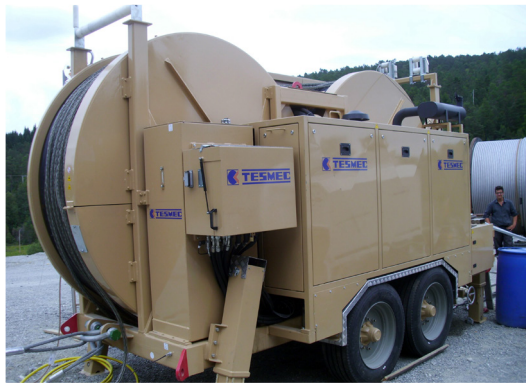
AFS804 BULL-WHEEL HUGE Ø Max Pull: 200 kN Bull-wheel Ø: 2400 mm Mass: 16000 kg
