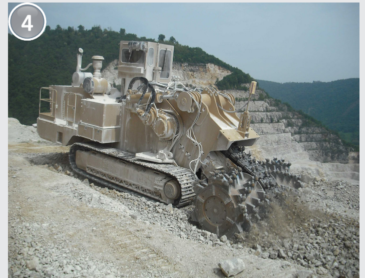
Picture 3 RH can work up-cutting and down-cutting by changing the attachment (hard rock excavation for foundations of building with 1475 RH down-cutting).
